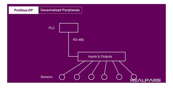
PROFIBUS DP (Decentralised Peripherals)[6] is used to operate sensors and actuators via a centralised controller in production (factory) automation applications.
