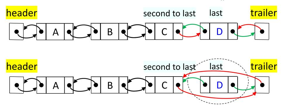
Here's a visualization of the code for removeLast().
