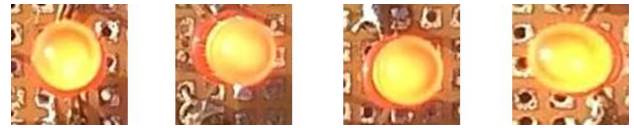
Fig. 4: The LED templates used for the classification by matching the KAZE features. The purpose of this matching is to find out which LED is ‘ON’ in order to decode the LED array pattern from the image.
