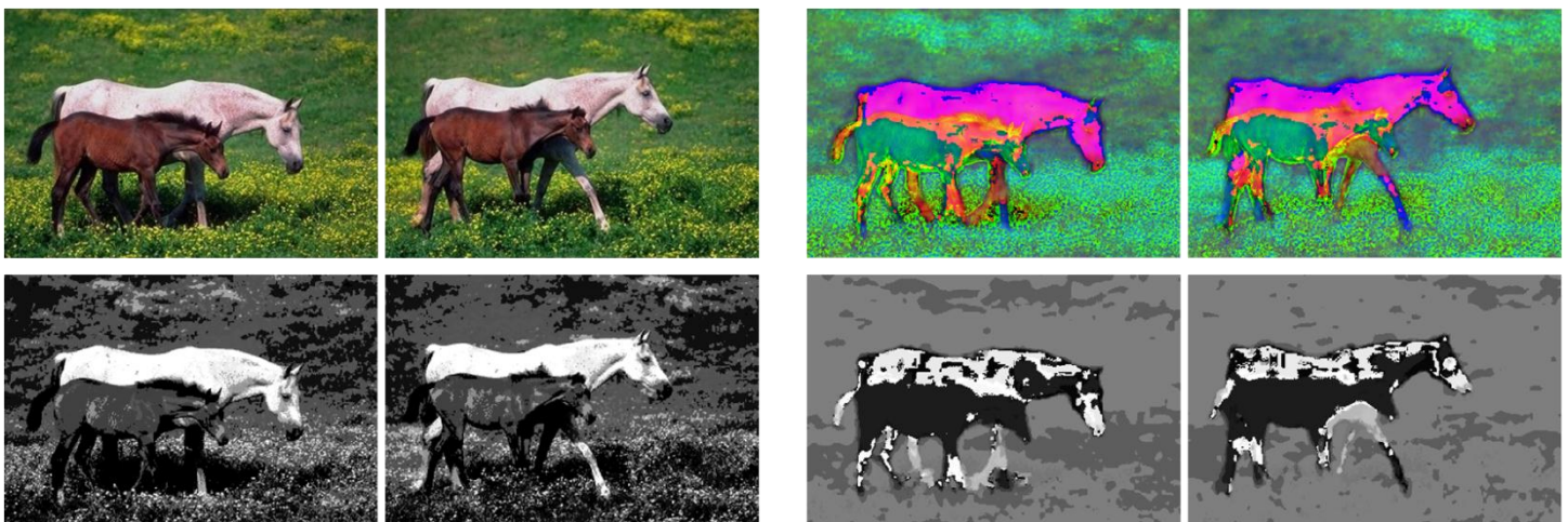
Fig. 12. Visualization of RGB (64 bins) and HSV (72 bins) color quantization. The first two columns shows RGB images and RGB quantized images and last two columns shows HSV images with HSV quantized images. It can be observed that last two images in the second row lost various details of the original image as compared to the first two images in the second row.
