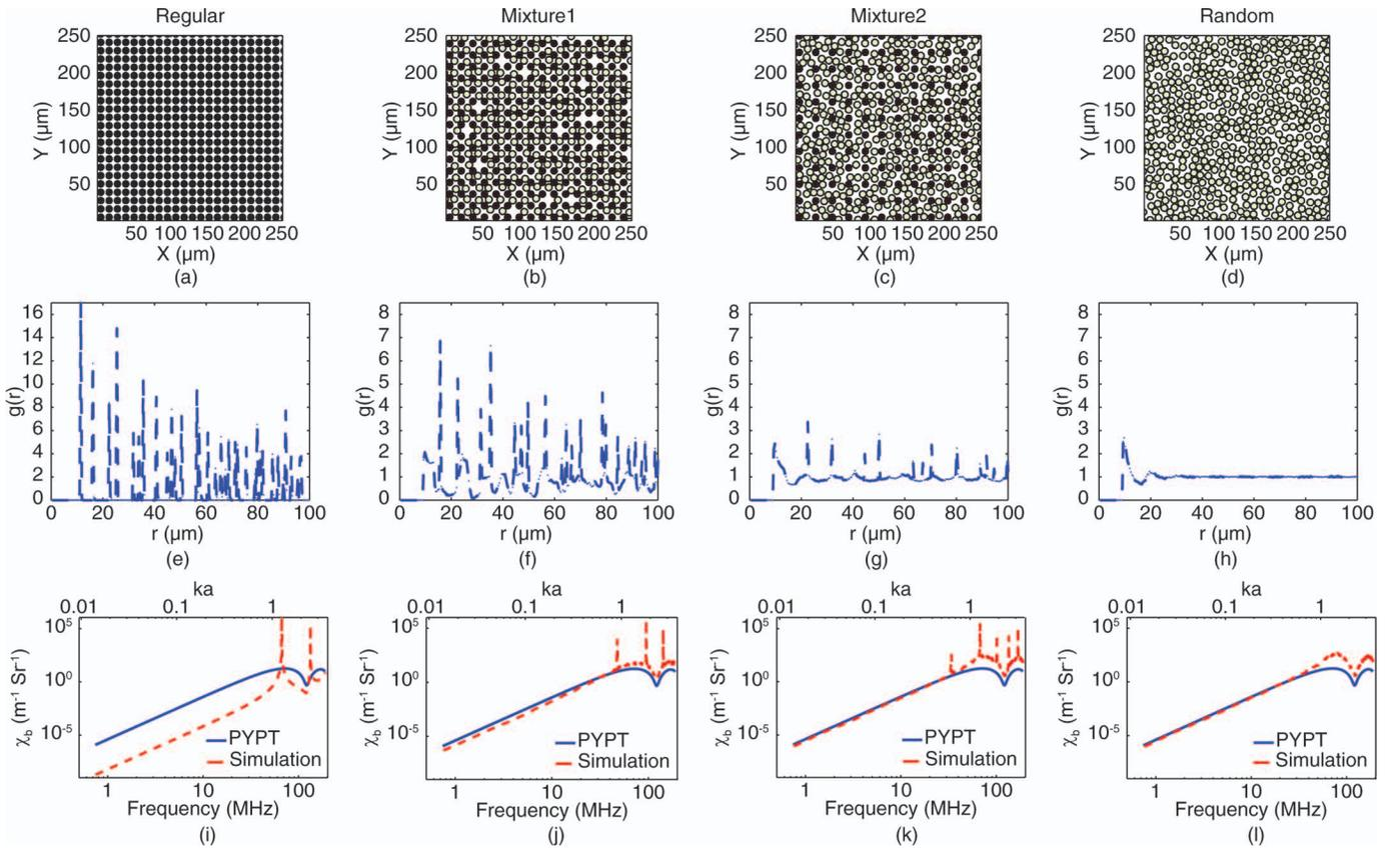
Fig. 2. (a) A tissue sample with regularly spaced nuclei. (b) and (c) Tissue samples with mixtures of regularly (dark circles) and randomly placed nuclei (gray circles). (d) A configuration of randomly packed nuclei. (e)–(h) Plot of pair correlation function for (a)–(d), respectively. (i)–(l) Frequency-dependent BSC for (a)–(d), respectively.
