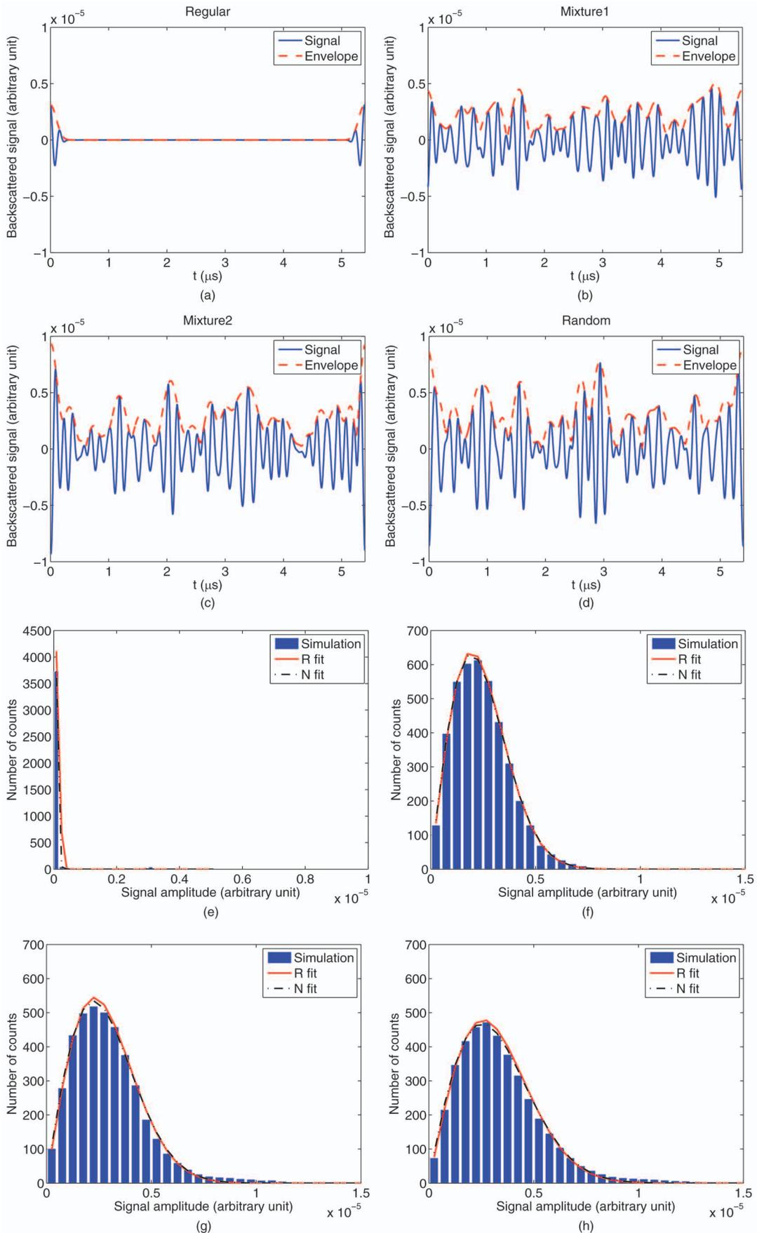
Fig. 4. (a)–(d) Representative signals from four different tissue samples. (e)–(h) Corresponding histograms for 100 RF lines and fitted with Rayleigh (R) and Nakagami (N) distribution functions.
