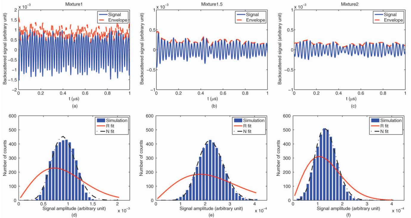
Fig. 5. (a)–(c) Simulated signals for Mixture1 (excited with 50-MHz pulse), Mixture1.5 (excited with 25-MHz pulse), and Mixture2 (excited with 25-MHz pulse). For clarity, a portion of the RF line is presented for each sample. (d)–(f) Corresponding histograms generated from 100 RF lines fitted with the Rayleigh (R) and Nakagami (N) distribution functions.
