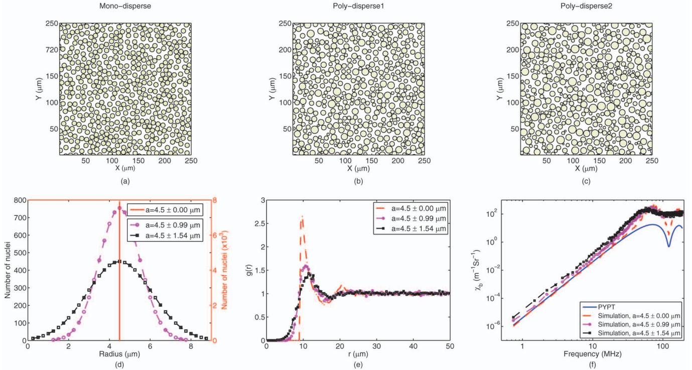
Fig. 3. (a) A random arrangement of mono-disperse nuclei. (b) and (c) are the same as (a) but for poly-disperse nuclei. (d) Variations of number of nuclei with radius for mono-disperse (solid line, right axis) and poly-disperse samples (broken lines, left axis). The mean ( $\pm 1$  standard deviation) values are given in the legends. (e) Plots of pair correlation function for three samples. (f) Variations of frequency-dependent BSCs for those samples.
