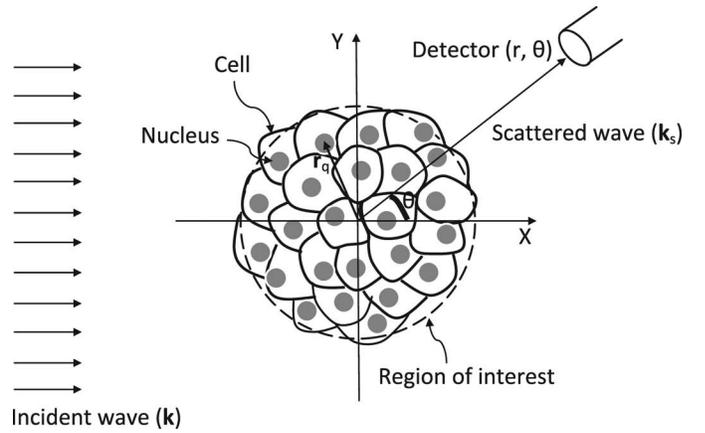
Fig. 1. Scattering diagram (top view). Here,  $\mathbf{r}_q$  is the position vector of the  $q$ th scatterer with radius  $a_q$  and  $\theta$  is the scattering angle. For backscattering,  $\theta = \pi$ .
