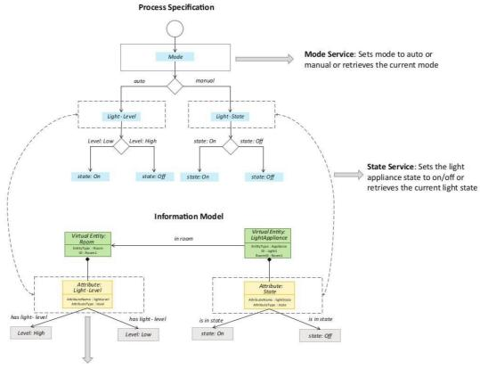
Controller Service: In auto mode, the controller service monitors the light level and switches the light on/off and updates the status in the status database. In manual mode, the controller service, retrieves the current state from the database and switches the light on/off.
