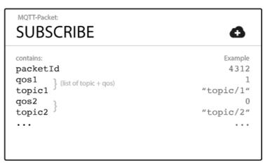
**Packet Identifier :** uniquely identifies a message as it flows between the client and broker. The client library and/or the broker is responsible for setting this internal MQTT identifier.
