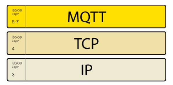
MQTT connection is always between one client and the broker. Clients never connect to each other directly
