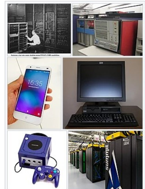
Computers and computing devices from different eras – clockwise from top left: Early vacuum tube computer ( ENIAC ) Mainframe computer ( IBM System 360 ) Desktop computer ( IBM ThinkCentre S50 with monitor) Supercomputer ( IBM Summit ) Video game console ( Nintendo GameCube )
