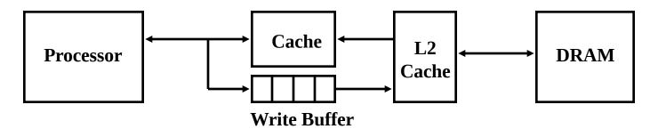
**Write-miss Policy: Write Allocate versus Not Allocate**
