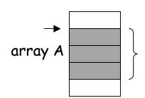
Initially \$s3, \$s4, \$s5 contains i, j, k respectively. Let \$s6 store the base of the array A. Each element of A is a 32-bit word.
