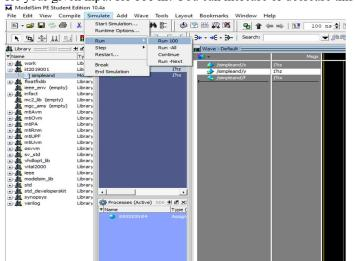
9. Repeat the steps 7 and 8 for different inputs and you will see the waveform in the wave window. ModelSim PE Student Edition 10.4a
