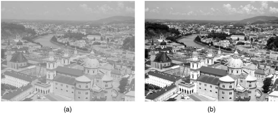
FIGURE 8.7 (a) Example of an image whose original gray-level range was [90, 162]; (b) the result of applying the autocontrast transformation (equation (8.4)).
