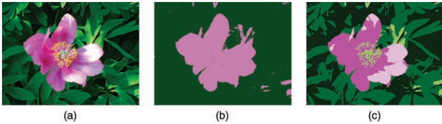
FIGURE 16.29 Another example of color segmentation using requantization: (a) original image; (b) requantized image with two color levels; (c) requantized image with five color levels.
