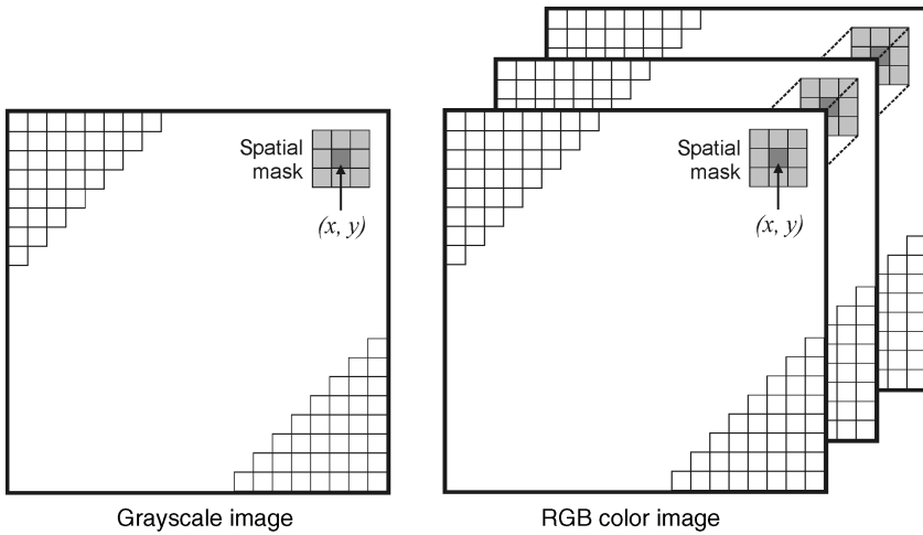
FIGURE 16.25 Spatial convolution masks for grayscale and RGB color images.
