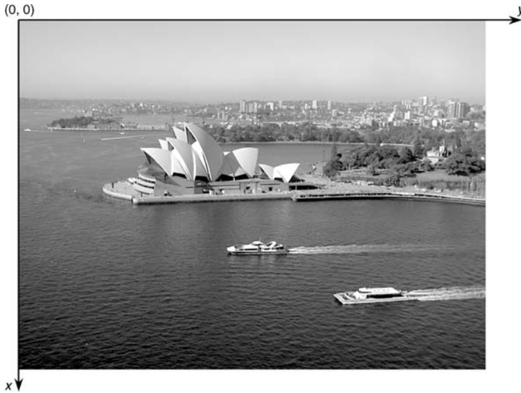
FIGURE 2.1 A monochrome image and the convention used to represent rows ( x ) and columns ( y ) adopted in this book.
