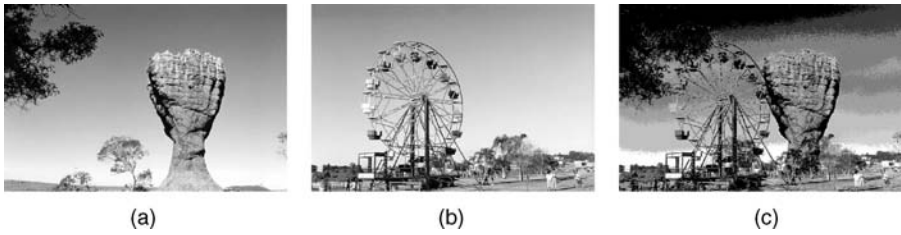
FIGURE 6.8 The AND operation applied to monochrome images: (a) X ; (b) Y ; (c) X \text{ AND } Y .
