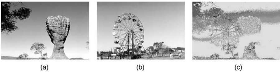
FIGURE 6.9 The OR operation applied to monochrome images: (a) X ; (b) Y ; (c) X \text{ OR } Y .
