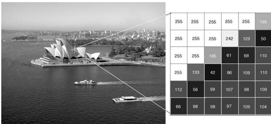
FIGURE 2.3 A grayscale image and the pixel values in a 6 \times 6 neighborhood.
