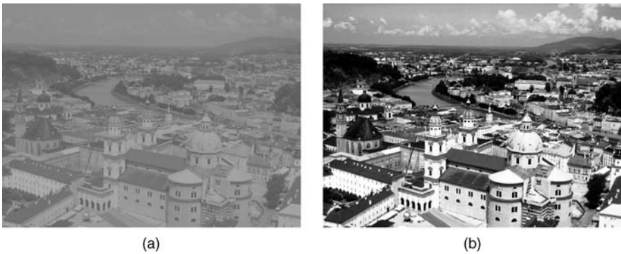
FIGURE 1.7 Contrast enhancement: (a) original image; (b) after histogram equalization to improve contrast.
