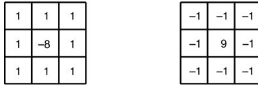
FIGURE 10.15 Laplacian masks that account for corner pixels (standard and composite).
