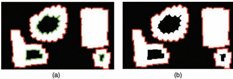
FIGURE 18.9 Tracing boundaries of objects and holes.
