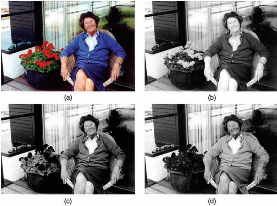
FIGURE 2.4 Color image (a) and its R (b), G (c), and B (d) components.
